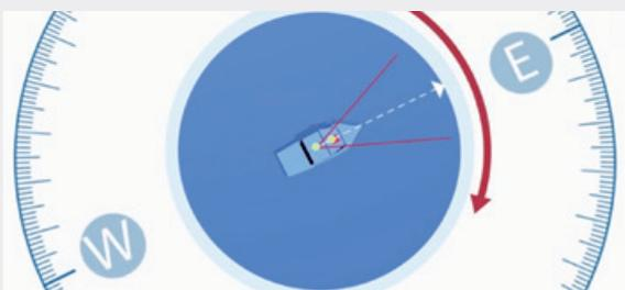
Dual antenna GNSS provides accurate heading with fast initialization time, even if the vessel is mooring. Additionally, it is not subject to latitude scaling faced by gyro-compass technology.
