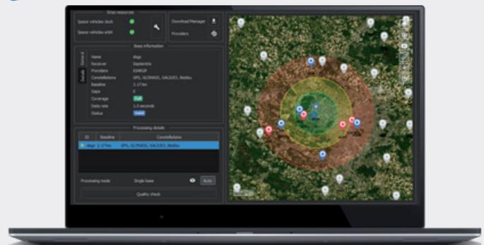
**Why Post-processing ?** By processing all your INS and GNSS raw data forward and backward, Qinertia PPK software greatly increases accuracy, solves GNSS outages, installation errors, etc. Qinertia can save your survey, or allow you to survey in very complicated areas.
